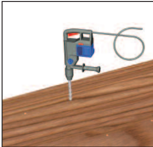
1: Stack standard 3/4" or 5/8" plywood sheets. Drill with 9/16" drill bit.
