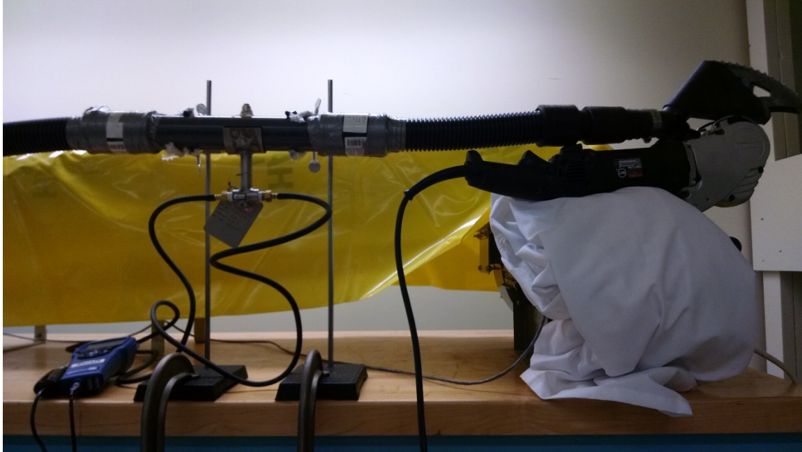
Figure 5 - Flow measurement set up
