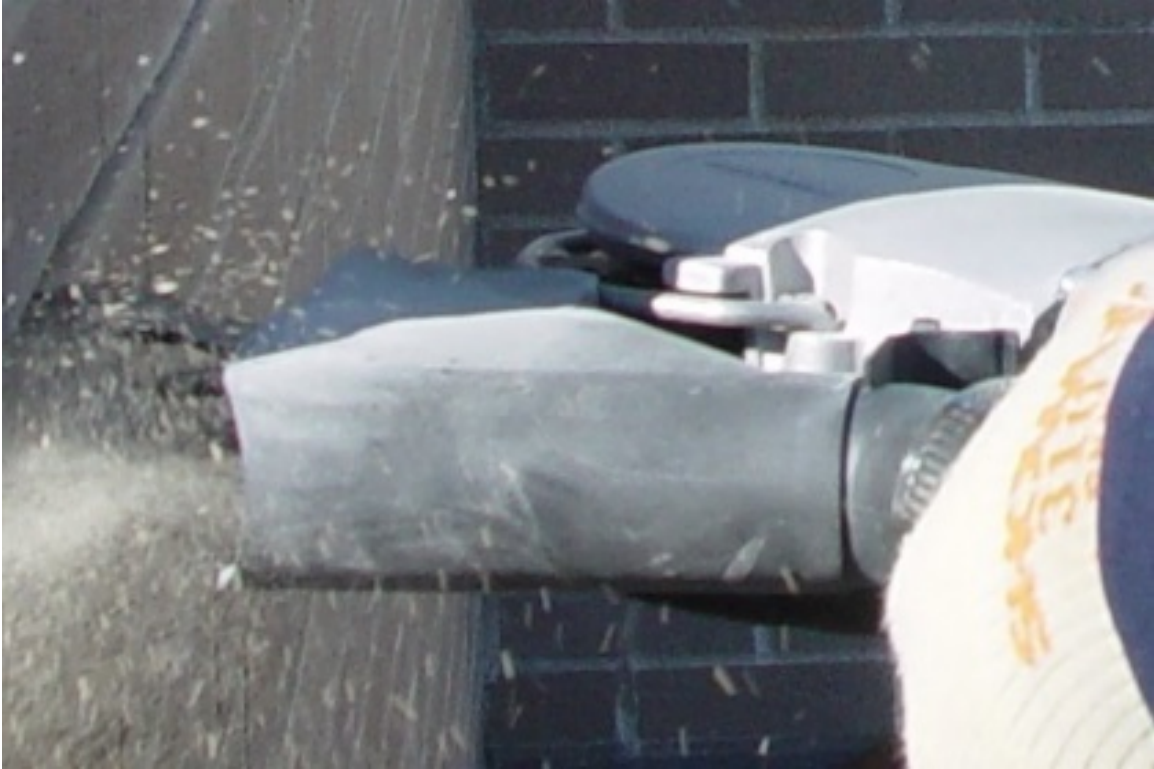
Figure 2 - Dust extraction hood in use (NIOSH photo)
