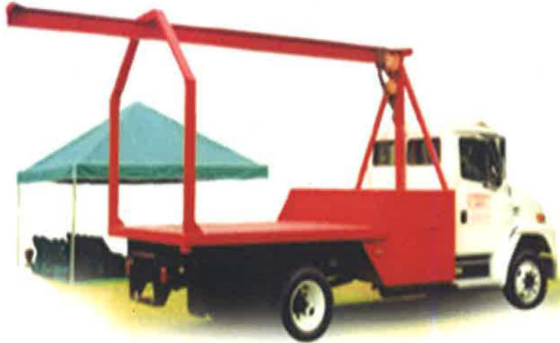
Photo 4: Burial Vault Delivery Rig
