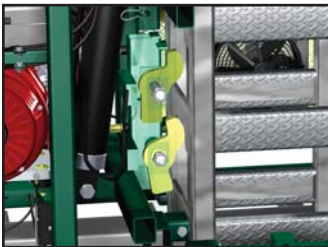
fig. 2.7 Safety hooks in normal working position
