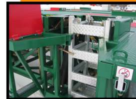
Open deck design to pass wall ties. New climbable tower w / quick connect bolts, no X-braces
