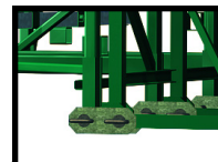
Bridge link plates and pins (8x)
