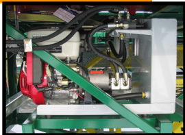
Simple hydraulic dual pump system w / reliable Honda 9.0 HP
