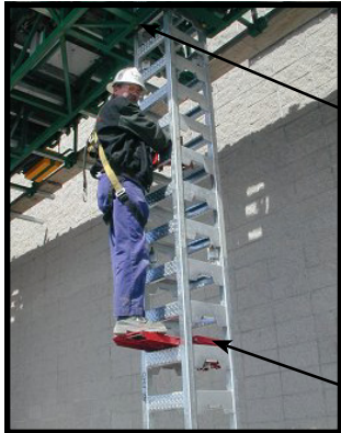
Automatically retracting rest platform
