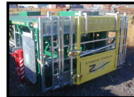
Build-in storage for guard rails and doors on motorized unit ends.
